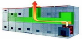
Figure 4 – Illustration of Arc Resistant Venting
