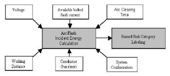
Figure 1 – Incident Energy Calculation
