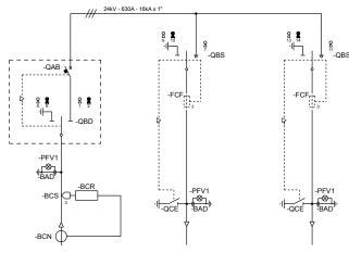
(\*) Motor-operated HySec includes the local/remote selector switch and opening and closing push-buttons
