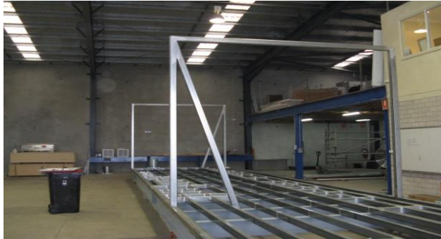
Base Frame – fully welded, custom designed to suit equipment loadings and cable penetrations
