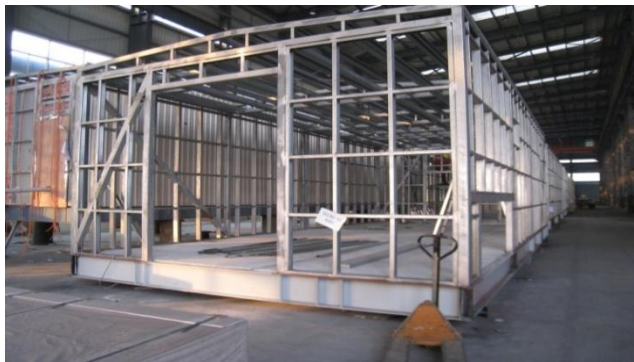
Walls & Roof Frame – fully welded or bolted sections.
